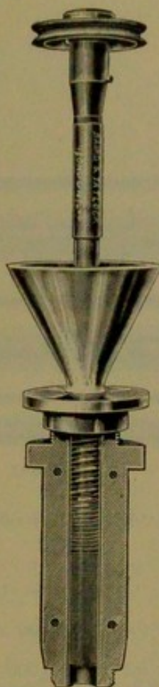
Section of screwed spindle in cylinder with funnel and driving pulley wheel
