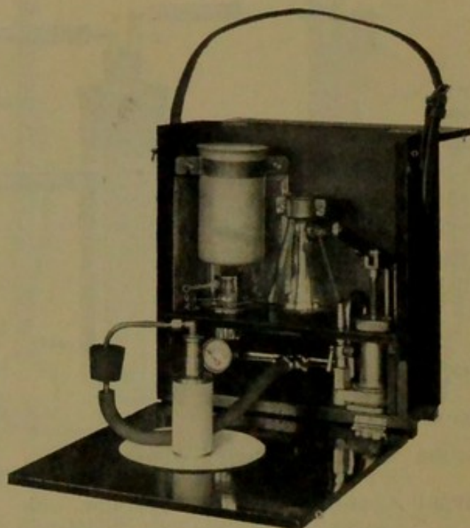
(2) Cleaning the Brass Filter by Reversal with Compressed Air.
