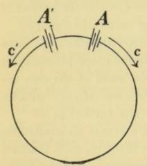
Let us consider two of these accumulators, A and A', inserted with their poles inverted in the same circuit. Suppose they are quite identical, except that the one, A', is entirely without charge, and the other, A, has its full charge. Let us suppose now that the current, c, generated by A which tends to charge A' can under certain circumstances cause an oscillatory discharge, i. e., a continuous oscillation of the current, now in the direction of c, now
