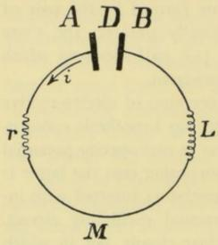
Let A and B be the armatures of a charged condenser which are suddenly connected with each other by an external conductor, ArMLB, in such a way that the latter makes a circuit open only at the point D of the di-electric. In the accompanying figure r represents the total resistance of the circuit, and L the inductance or coefficient of self induction of this circuit. When the capacity c of the condenser and the inductance L of the circuit are in a certain
