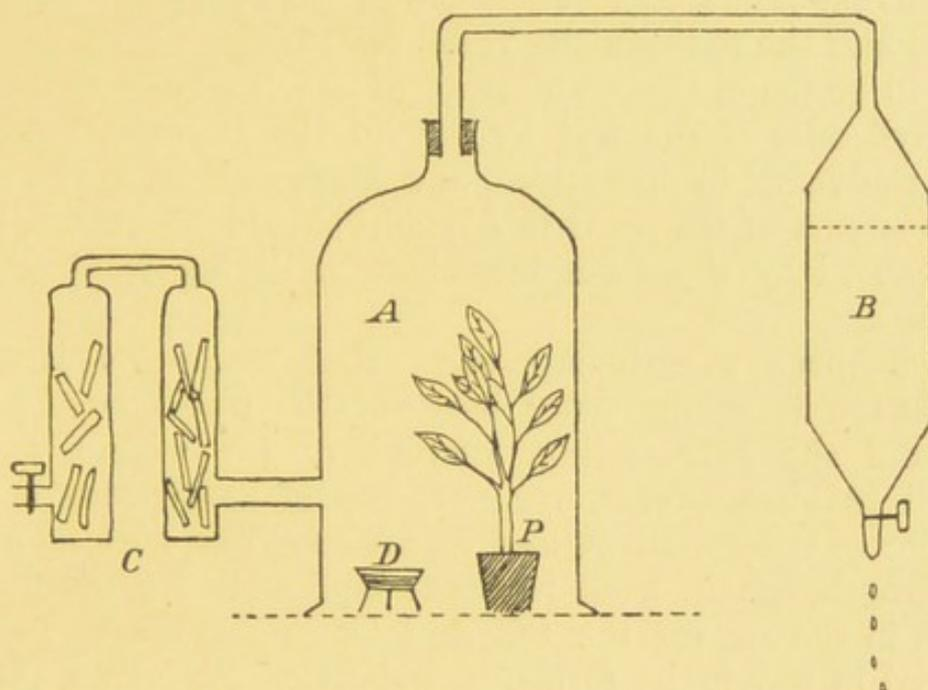
Fig. 114.—APPARATUS FOR DEMONSTRATING THE EVOLUTION OF  $\text{CO}_2$  FROM A PLANT DURING RESPIRATION.—A, Large bell-jar; P, plant; D, small dish containing a saturated solution of caustic potash; C, tubes containing sticks of caustic potash to absorb the  $\text{CO}_2$  of the atmosphere before it is drawn into the jar A; B, aspirator.
