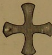
Screw-calk with + -formed cross-section (patented by Gück).
