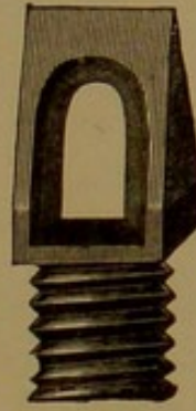
Perforated calk of A. Lungwitz.
