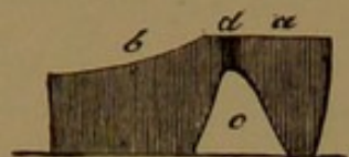
Transverse section of a branch of a front shoe: a , bearing-surface; b , concaving; c , fullering, or "crease"; d , nail-hole.
