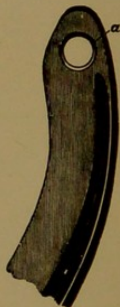
Ground-surface of the end of a branch of shoe, showing (a) hole and counter-sinking for a screw-calk (one-half natural size).
