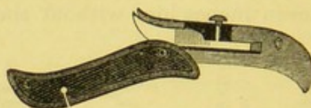
FIG. 488.—THE SAME, WITH ONE SIDE OF THE HANDLE MOVED OFF TO SHOW THE MANNER IN WHICH THE BUTTON ACTS ON THE SPRING.
