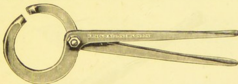
FIG. 624.—COMPRESSION FORCEPS, FOR ASCERTAINING THE SEAT OF PAIN IN THE HORSE'S FOOT.
