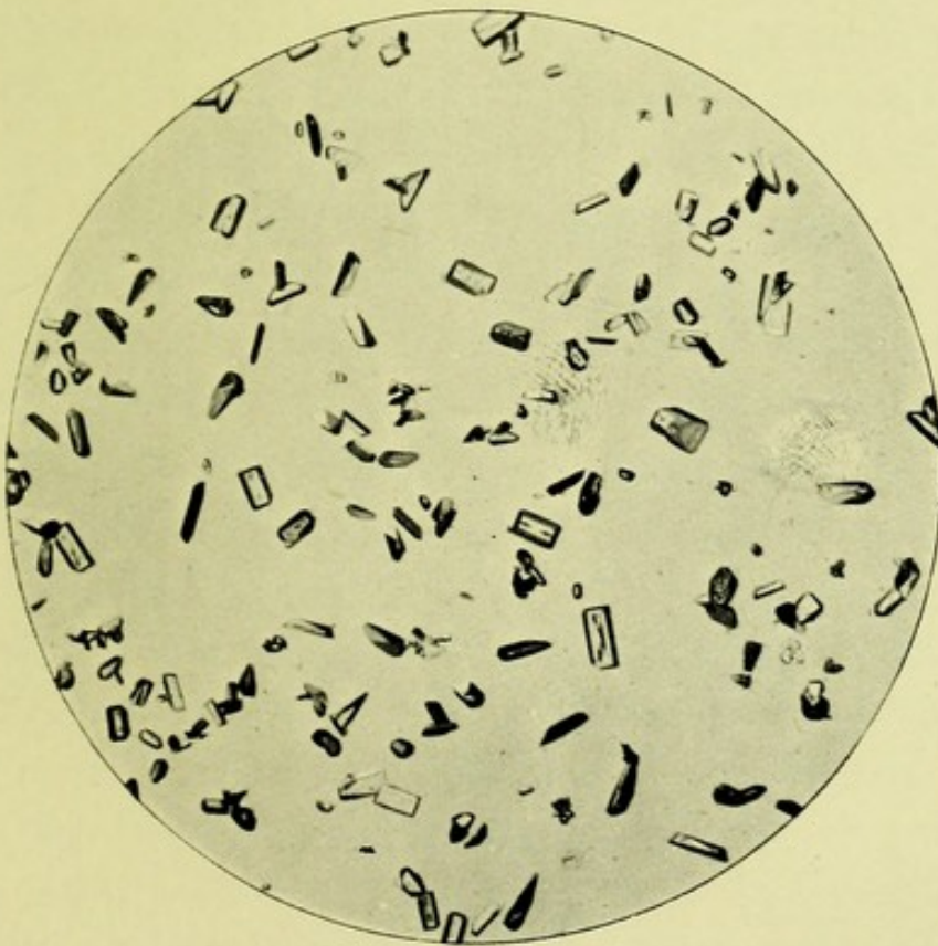
FIG. 29.—Rhombic Crystals of Ammonium Magnesium Phosphate, showing Special Growth along Line of Scratch.
