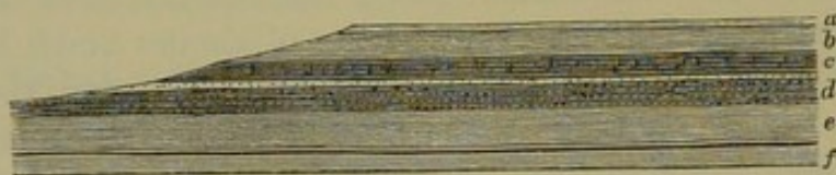
FIG. 104. Section of Round Hill, Landsdown, near Bath (reduced from the Geol. Survey). a. Great Oolite. b. Fuller's-Earth. c. Inferior Oolite. d. Marlstone. e. Lias. f. New Red Sandstone.
