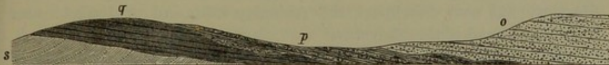
FIG. 64. Section across the south end of the Coalbrookdale Coalfield, near Bridgenorth, showing the unconformity between the Carboniferous and Permian, and between the Permian and Trias. (Reduced from the Geol. Survey.) o. New Red Sandstone. p. Permian. q. Coal-measure. s. Old Red Sandstone.
