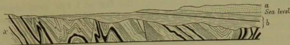
FIG. 15. Section across the Rivière du Nord. (Logan.) a. Potsdam Sandstone. b. Acadian Rocks, with track-bed in centre. x. Archæan Gneiss with limestone and dykes of trap and granite.
