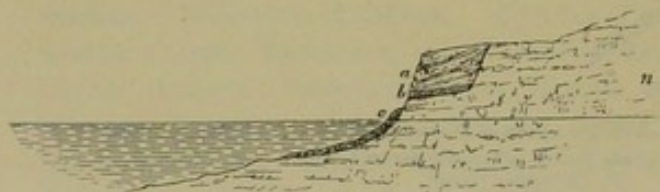
Fig. 249*. Diagram-section across the coast east of Brighton. a. Elephant-bed (head or rubble). b. Raised beach. c. Present beach. n. Chalk.
