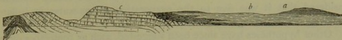
FIG. 71. Section through the Carboniferous Limestone anticlinal five miles N.W. of Bristol. (Reduced from Geol. Survey, sect. 4.)
