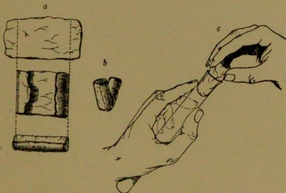
FIG. 24.—Plugging test-tubes: a , cylinder of wool being rolled; b , cylinder of wool being doubled; c , cylinder of wool being inserted in tube.
