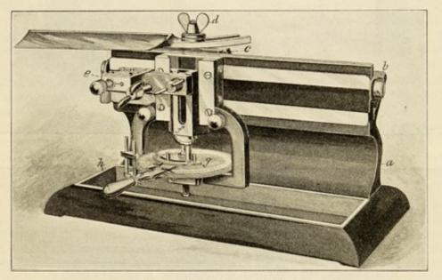
Fig. 4.-Laboratory microtome.
