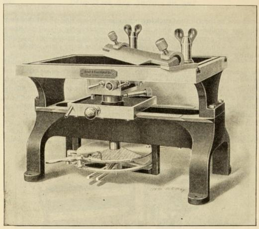
Fig. 5.-Minot automatic precision microtome.
