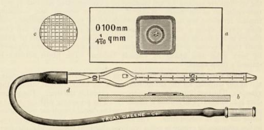
Fig. 179.—Thoma-Zeiss hemocytometer: a, Slide used in counting; b, sectional view; c, a portion of ruled bottom of the well; d, pipette.
