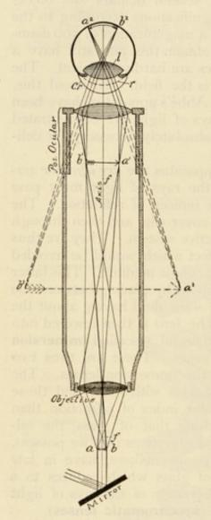
Fig. 2.—Diagram showing the principle of a compound microscope with the course of the rays from the object  $(a \ b)$  through the objective to the real image  $(b^1 \ a^1)$ , thence through the ocular and into the eye to the retinal image  $(a^2 \ b^2)$ , and the projection of the retinal image into the field of vision as the virtual image  $(b^3 \ a^3)$ .—(Fig 21, Gage, The Microscope, eighth edition.)
