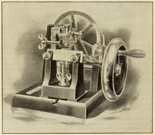
Fig. 6.-Minot automatic rotary microtome.
