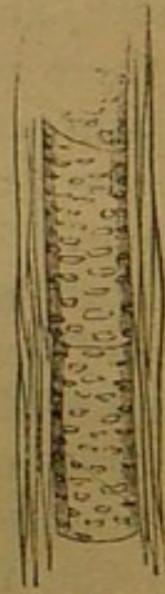
FIG. 63. Thin section of Oak-wood, magnified, showing a dotted vessel, between long wood-cells.
