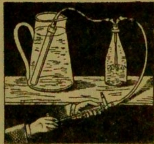
FIG. 6. — Berkefeldt's Filtering Apparatus, complete, with porous cylinder, vacuum flask, india-rubber stopper, and exhaust pump.
