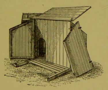
FIG. 6. THE VERO SHAW KENNEL, SHOWING SECTIONS.
