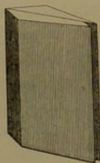
FIG. 44.—Perspective view of Jellett's analysing prism.
