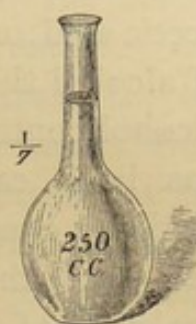
FIG. 34.—Measuring Flask, holding the quantity marked on the body of the flask when filled up to the circular mark round the neck.
