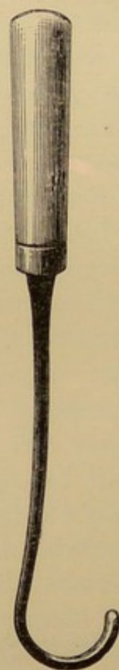
FIG. 14.—Hook-shaped gouging chisel for producing grooves for grafting.
