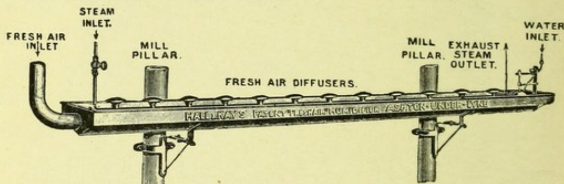
FIG. 7.—Humidifying trough as used in yarn conditioning cellars. Hall & Kay, Ltd.
