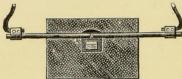
FIG. 50.—MOISSAN'S ELECTRIC FURNACE (CROSS-SECTION).
