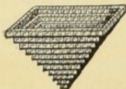
FIG. 63. — HOPPER-CRYSTAL OF SALT.
