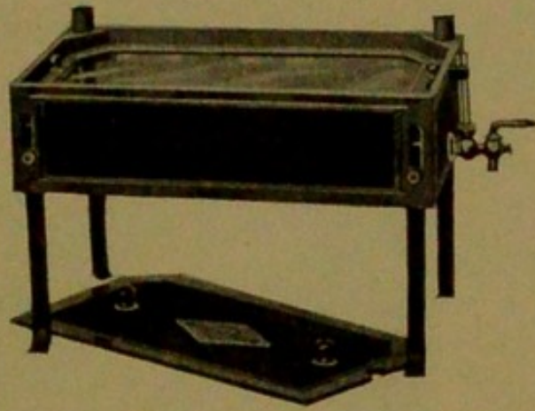
FIG. 89. Inspissator, for the sterilization of media at temperatures below the boiling point of water.
