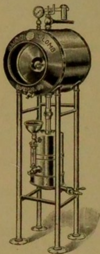
FIG. 88. Autoclave for sterilizing in live steam under pressure.
