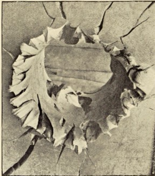
Fig. 9. —Another splash produced by projectile on armour plate (plan).
