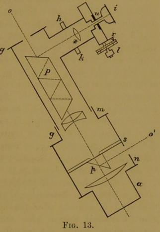
which the light from the objects serving for comparison-spectra falls upon the prism and is totally reflected through the series of prisms above to the eye of the observer at o. This apparatus may be used for observing the spectrum of the Algæ chlorophyll-green placed on the microscope-stage, and simultaneously the comparison-spectrum of a solution of chlorophyll in alcohol in a small test-tube placed in front of the aperture at o' on a specially devised stage.
