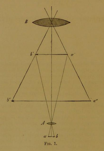
mined by  $p_1$ ,  $p_1$  by  $p^*$ , and  $p^*$  by p, and, consequently, the first quantity  $p_1^*$  by the last p. It is always possible, therefore, so to regulate the distance of the object from the objective that the final virtual image shall be at the distance from the eye of distinct vision.
