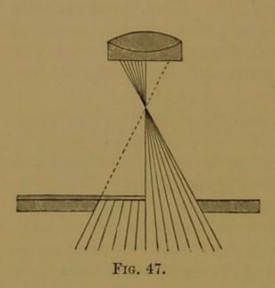
for the resolution of difficult details, consists of an incident cone of light, whose axis is more or less inclined to that of the Microscope. Such a cone may be obtained by placing the mirror or the diaphragm somewhat laterally to the optic axis, or by covering up a portion of the diaphragm, so that merely half, for instance, of the original cone is effective (Fig. 47). It is evident that if the angle of aperture of the diaphragm were equal to that of the
