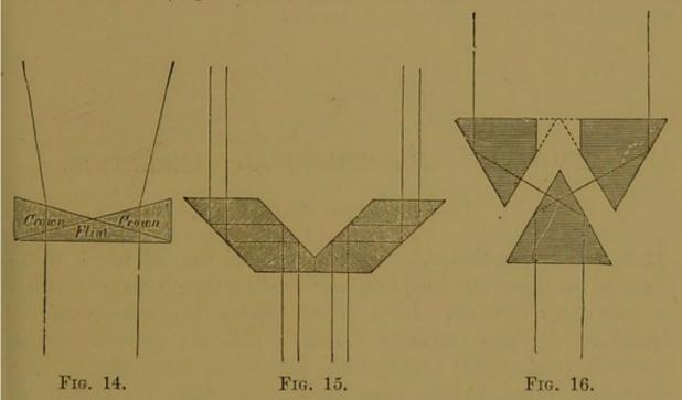
prisms in dividing the pencils into two parts is evident from the construction; it is also obvious that if in Fig. 16 the upper prisms (or the faces at which the second reflexion takes place) are turned round 90° a complete reinversion of the objective-image must be caused. The optician has it therefore in his power to give an erect or an inverted position to the final virtual image.
