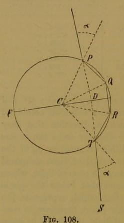
triangles C P Q, C Q R, and C R T are similar, and their angles adjacent to the chords P Q, Q R, and R T are = a'. Consequently the three angles P C Q, Q C R, and R C T at the centre are together = 3 (180° - 2 a'). On the other hand, the triangle P C D gives the relation
