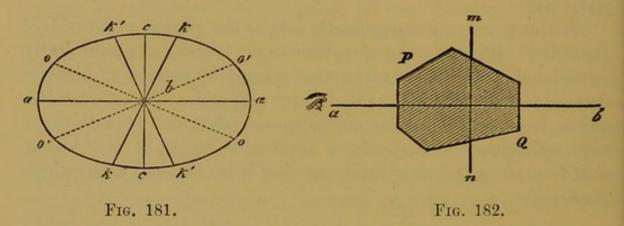
axis, which is perpendicular to the surface of the paper, appears therefore at b as a point. Let the two circular sections be k k and k' k'; they are also perpendicular to the surface of the paper, and are consequently seen as lines which form right angles with the normals o o and o' o'.
