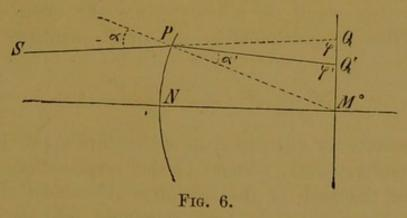
Q. Let the angles which this makes with P Q and P Q' be  $\phi$  and  $\phi'$ , and the angles of incidence and refraction  $\alpha$  and  $\alpha'$ . In the triangles P Q  $M^0$  and P Q'  $M^0$ , since P  $M^0 = r^0$ , the trigonometrical ratios are
