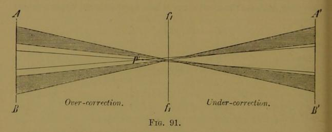
of this, the fog appears bluish, and the disc of light has a greenishyellow border, red at the extreme edge, which appears, up to a certain limit, the more decided the greater its diameter. The distinction between under-corrected and over-corrected aberration is thus still further facilitated.
