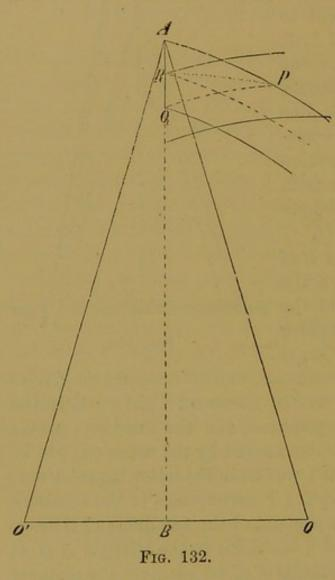
reflecting surface. They all lie in an arc drawn from Bthrough P, which, on account of the minuteness of the distances, is to be regarded as a straight line, and is therefore entirely in the plane of adjustment. The interference lines, if observed by homogeneous light, accordingly appear equidistant from one another by the magnitude  $\frac{a}{2d}\lambda$ . They therefore approach the nearer, the greater  $\phi$  is, i.e., the further the slit is from the reflecting-plane, and, when d =
