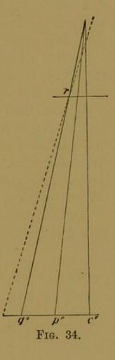
intersect in the centre of the field of view, must therefore appear in the image as straight lines; in every other direction, however, an irregular magnification involves their curvature, which is the stronger the greater their distance from the centre.
