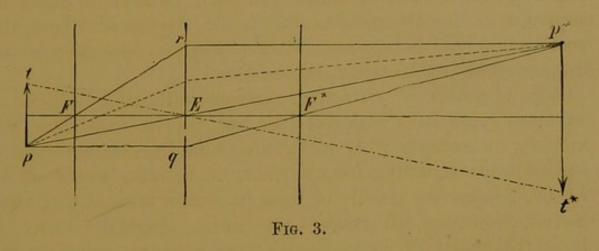
rays, which, after refraction, unite at  $p^*$ , and as all the other rays which proceed from p are refracted in a like manner to  $p^*$ , the image of the point p is formed at  $p^*$ . By a similar construction the image of the other extremity t, as well as of all other points between p and t, may be obtained. To simplify the matter still further we can replace one of the two lines by the ray of direction  $p \to p^*$ , which passes through unrefracted.
