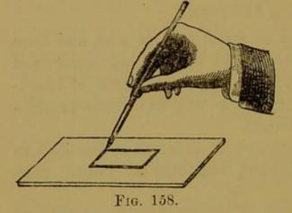
ridge of cement has partially dried, the preparation is placed in the enclosed space, and the latter is filled with the preservative fluid selected. If we have added too much of the fluid, the excess can be easily removed with a brush. It is convenient to put the
