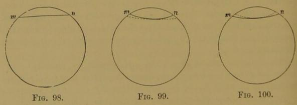
an object, is made to coincide with this chord precisely as the adjustment of a particular division-line to the margin of an object is effected in micrometric measurements. If a complete coincidence takes place—whether or not they appear straight or curved in the virtual image—then the real image is free from distortion; in all other cases it is distorted.
