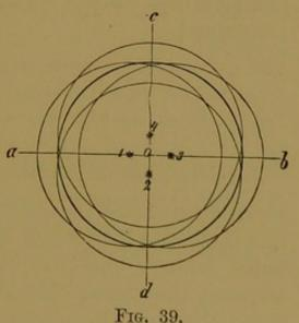
be extended. It therefore describes a circle, of which the point o is the centre, and the distance of the displacement is the radius. Similarly, every other point in the image (since its position relative to the centre must remain the same) describes a circle of equal
