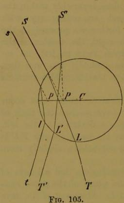
The centre itself is illuminated by rays which traverse it without refraction.
