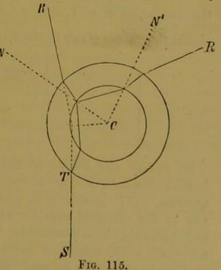
of the angles of aperture  $\omega$  and  $\delta$ , the thickness of the wall, and the refractive power of the different media. For the determination of the latter by a formula which will be generally valid, the following consideration may be utilized. If the ray S T (Fig. 115), incident from below, were, as in the previous case, reflected at the inner wall, the angle of deviation of the ray emerging towards R' would be given by the equation
