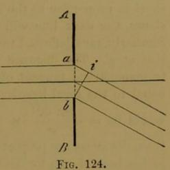
ing now the breadth of the transparent portion a b = 1 mic., and the wave-length of the incident light (considered to be homogeneous) =  $\cdot 5$  mic., then we get for the quantity a i the proportion
