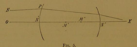
$r^0 = M^0 - N^0$ , r' = M' - N' (which values will therefore be positive for convex refracting surfaces and negative for concave), the equation for the incident ray assumes the form
