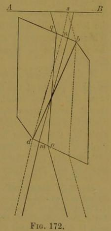
the most favourable circumstances. The two lines m n and p q represent two limiting rays, which pass through the prism in the directions determined above, and suffer the deviation figured at
