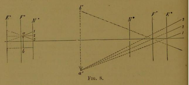
Fig. 8 shows how the last paths of the rays are to be constructed in such a system; a b is the object and a' b' the virtual image. The lines indicated by 1, 2, 3 correspond to each other; they cut the principal planes  $E^0$  and  $E^*$  at equal distances from the optic axis, and their direction is determined by the familiar laws of refraction.
