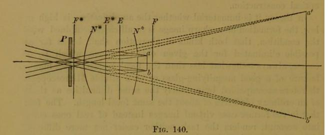
incident cones of light consequently being equal to the principal planes of the pupil, then the angle of aperture  $\omega$  is obviously determined for the middle of the field of view by the formula
