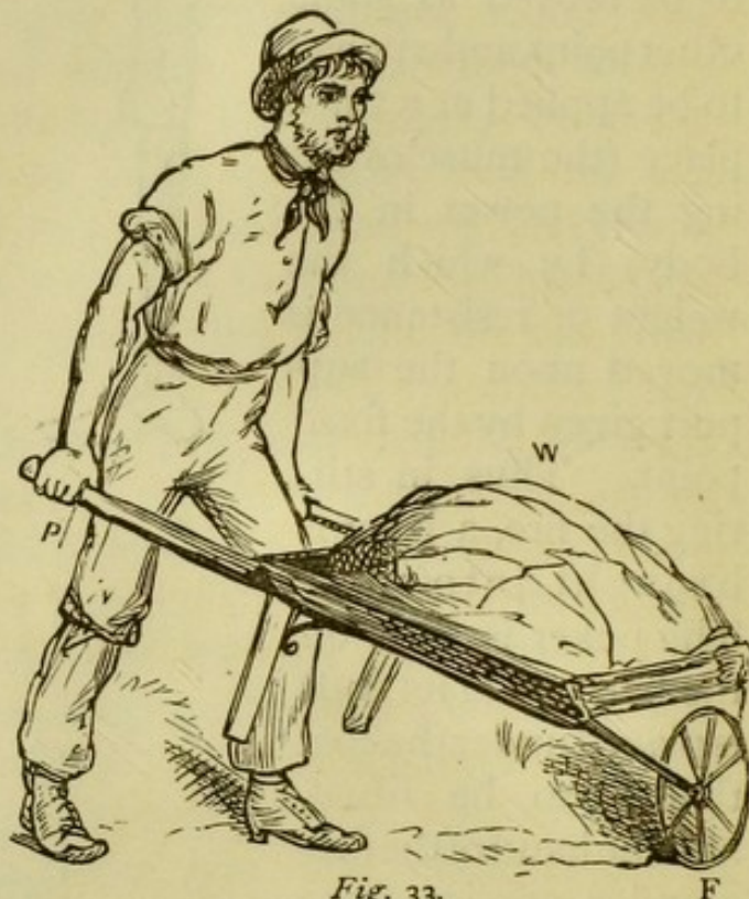
Fig. 32.—A LEVER OF THE SECOND ORDER.
