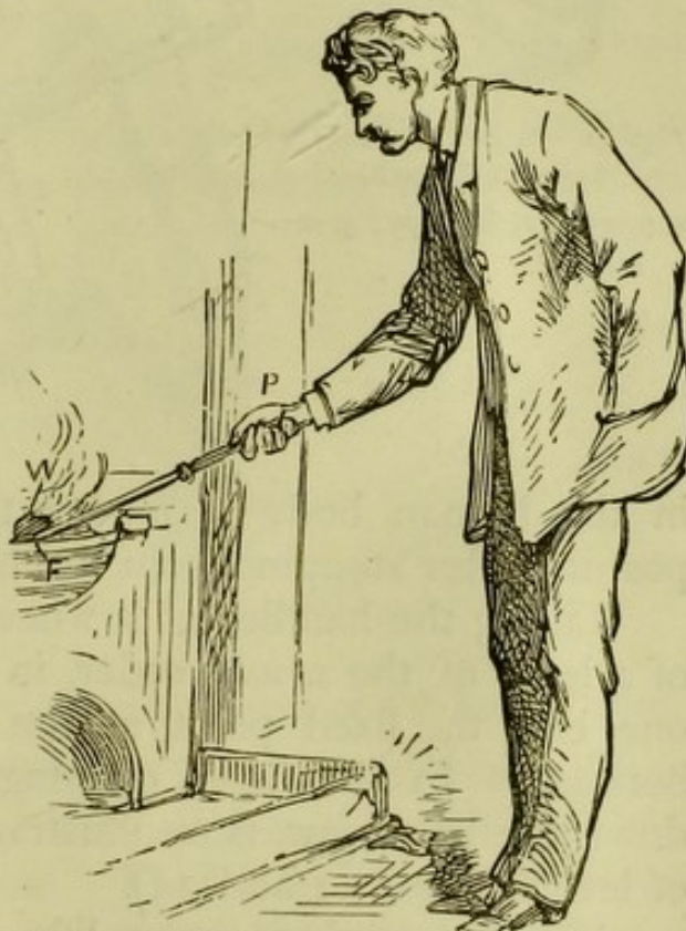
Fig. 31.—A LEVER OF THE FIRST ORDER.
