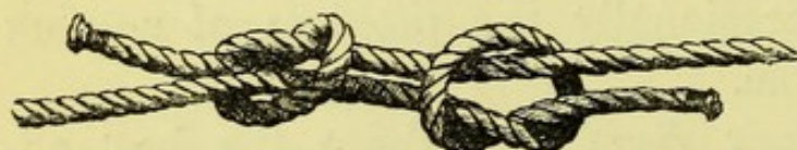
FISHERMAN'S BEND (For joining two ropes.)
