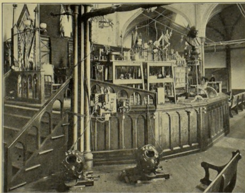
FIG. 22.—Three H.P. Motor and Generator supplying Bank of Lamps and operated by shielding with the hand a Selenium cell from an Acetylene Flame.
