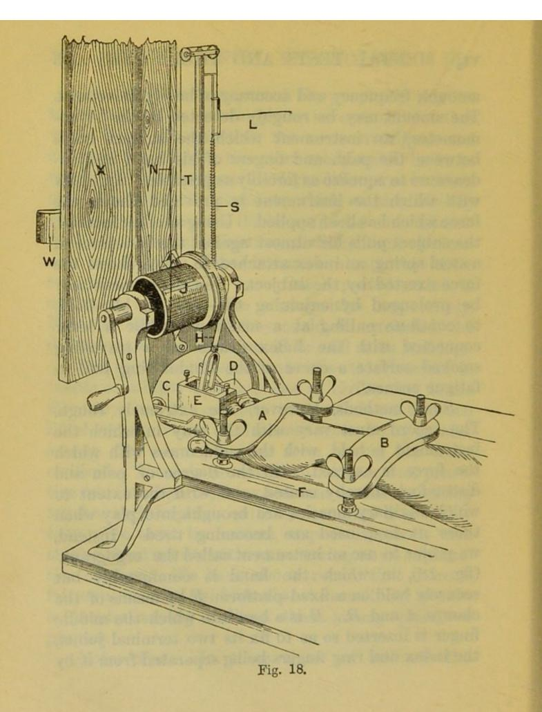
the plates C and D. The hand and arm are thus fixed so that only up and down movements of the middle finger at the knuckle joint are possible. These movements are communicated to the spirally grooved cylinder J by means of the steel ribbon H. To this cylinder is attached a wire N which passes over a pulley at the top of the board X, 10 feet or more in height. The other end of the wire falls behind this
