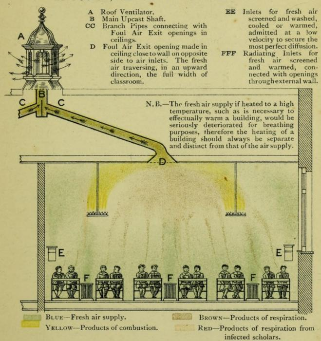
"Science proves that there is not a moment of time but when there is a movement of the air, and that this movement properly utilised is sufficient at all times to change the air in a building and secure ventilation."
