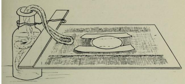
Live slide for the continuous observation of ameebæ in solutions of constant strength. The ameebæ are placed on the cover-slip, which is prevented from pressing on the glass plate underneath by the interposition of two strips of thin paper. The solution slowly circulates from the bottle along the wick to a piece of linen on the glass plate and prevents the preparation from drying up.
