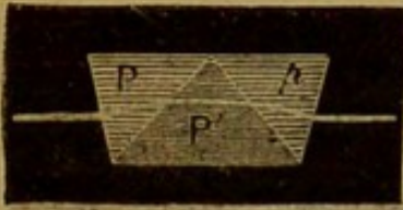
Fig. 27.—Amici's direct-vision compound prism.
