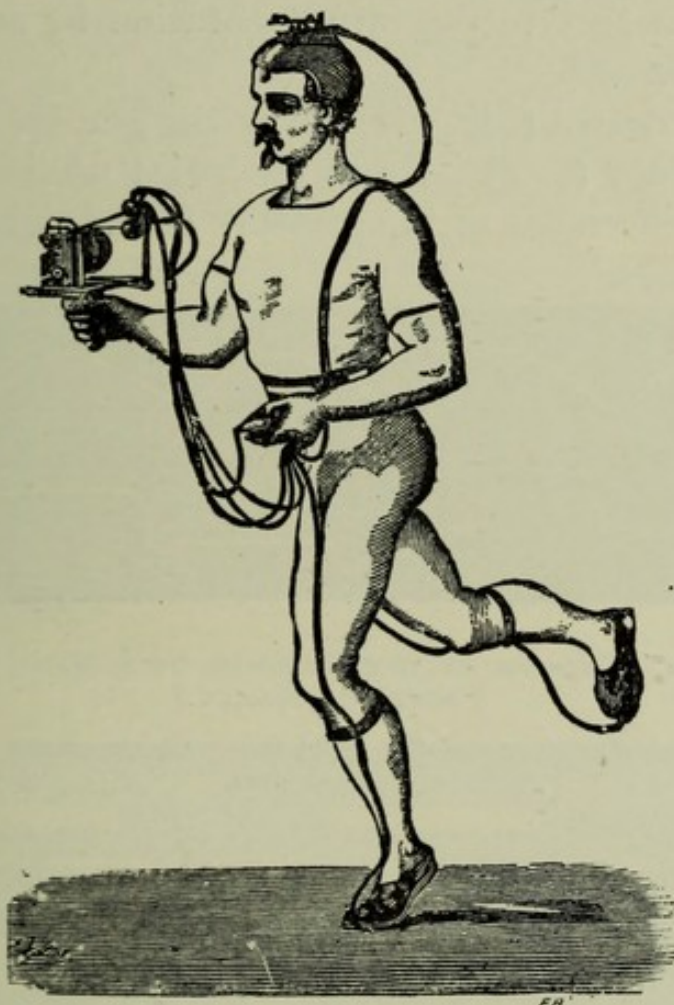
FIG. 116.—RUNNER FURNISHED WITH THE EXPLORATORY AND REGISTERING APPARATUS OF THE VARIOUS PACES.
