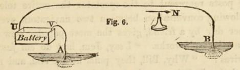
passes from the positive pole of the battery U, traverses the wire of the North-Western Railway, and after working the telegraph in Liverpool, descends into the earth by the wire B, which has a metal or earth-plate attached to it. From this point the electric fluid starts homewards, through the solid ground, and finding out the earth-plate\* under the foundations
