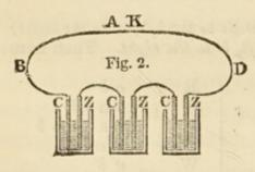
electric force, is combined with others, as in figure 2,—the zinc plate of one **D** cell being connected with the copper plate of the next by a piece of wire we shall have the celebrated battery invented by Volta in 1800, in which
