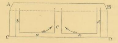
On the ground a wooden launder or pipe a a from 10 to 16 inches square, having the top perforated, is
