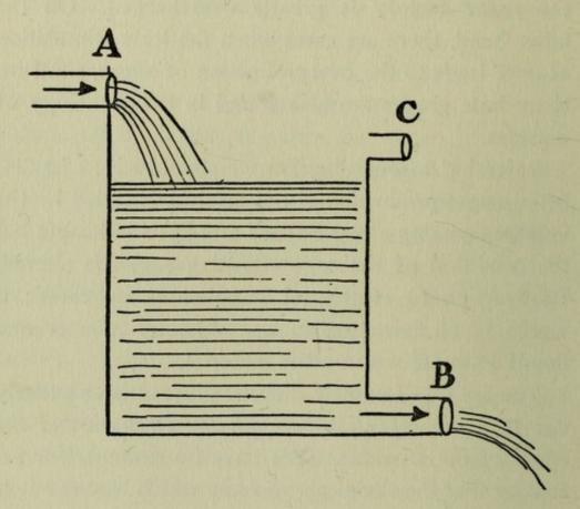
Imagine an open vessel, filled nearly to the brim with water. It has an escape pipe B, through which the water constantly flows out, while an equal quantity flows in at the supply pipe A. Thus the surface of the water always remains at the same height. If the conditions are altered and the vessel overflows, this may be due to several things.
