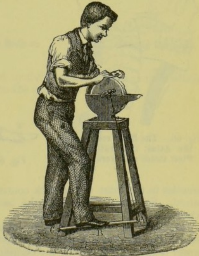
Fig. 65.—The Treadle, illustrating a Lever of the Third Order.
