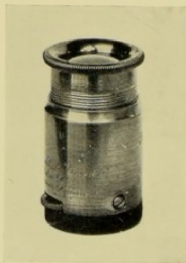
FIG. 11. The Spinthariscopes of Sir William Crookes.
