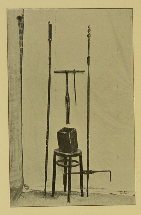
FIG. 1.-Photograph of Soil-sampling Tools.
