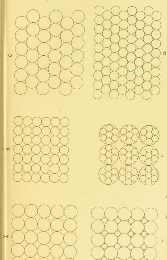
FIG. 2.-Diagram illustrating Pore Space between Spherical Particles.
