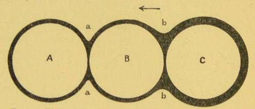
FIG. 5.-Diagram illustrating Liquid Film round Soil Particles.
