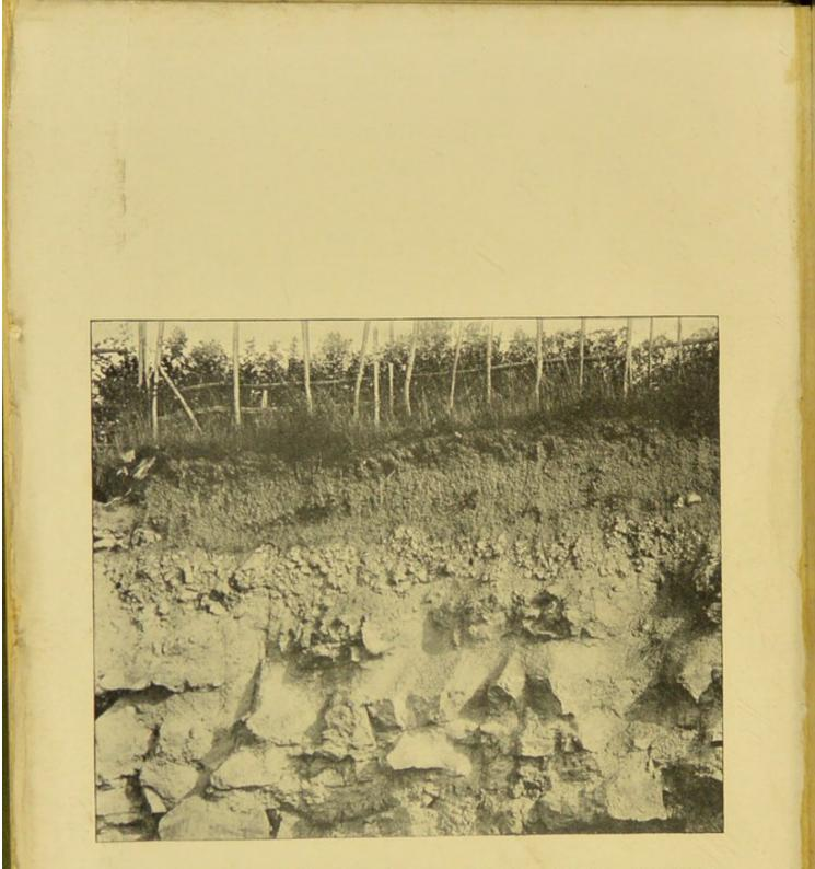
Photograph showing transition from Rock into Subsoil and Soil by Weathering (Hythe Beds, Great Chart, Kent).
