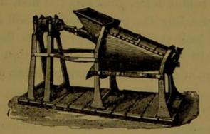
This machine is very useful to large makers for extracting pips, stalks, stones, &c., from raspberries, strawberries, currants, plums, apples,
