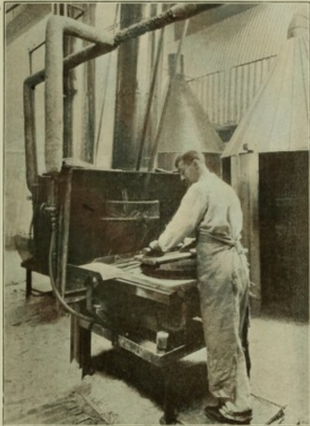
DIPPING TABLE AT BRYANT AND MAY'S FACTORY. SHOWING ARRANGEMENT OF BLOW-PIPE AND FAN, AND METHOD OF PRELIMINARY DRYING DIPPED SPLINTS.
