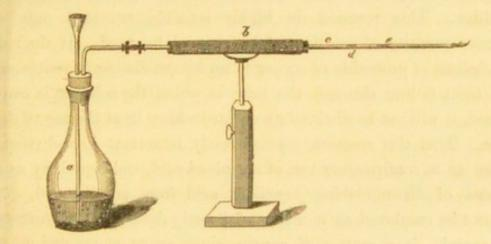
a is the evolution flask, b a tube containing chloride of calcium, c the tube in which, at the point d, the glass splinter with the specimen is placed. This part is then (the apparatus being completely filled with pure hydrogen gas) exposed to a slight heat, at first, in order to expel all moisture, and then suddenly to a very strong heat, (this is best done with a blow-pipe,) to prevent the sublimation of undecomposed sulphuret of arsenic. The metallic mirror is formed near the point e.
