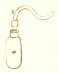
may be used, which in fact is more convenient than the glass tube c. a is the body of the gas bottle, into the neck c of which is ground air tight, the bent tube b, for conveying the gas into any inverted vessel. The bottom of the body a being made round and of thin glass, will bear a moderate heat, without the risk of cracking.
