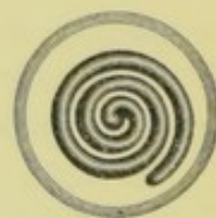
FIG. 40.— Spiral reservoir of mercurial surface thermometer.
