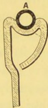
FIG. 77.— Section of Basin Rim with india- rubber pack- ing, A.
