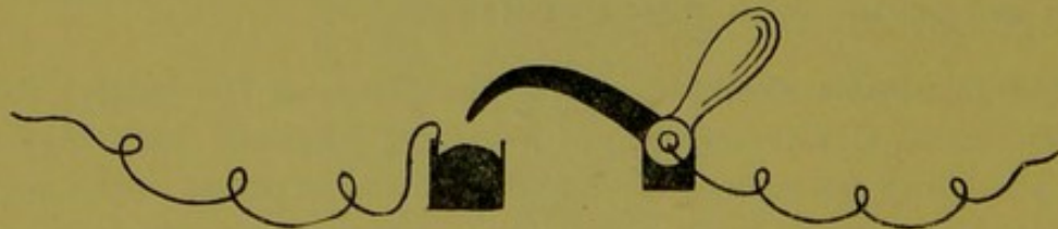
FIG. 9.—DIAGRAM OF MERCURY KEY.
