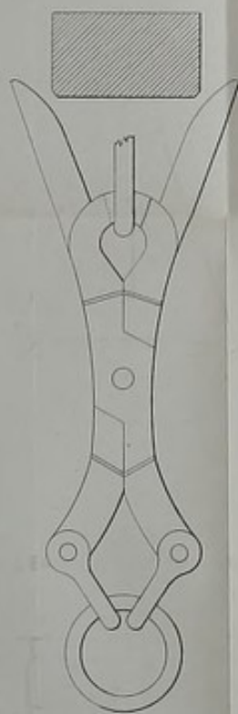
DISCONNECTING HOOK, FOR THE PREVENTION OF OVER WINDING.
