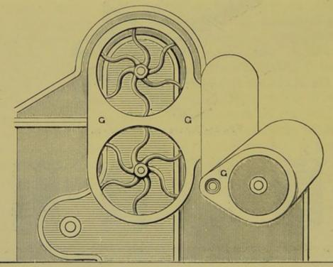
FIG. 11.—Spur wheels with suitable guards (G, G). (The arms of wheels may be covered with discs if needed).
