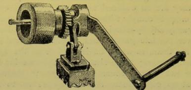
FIG. 2.—Safety starting-gear for gas and oil engines. The gear can be attached to either end of the shaft.
