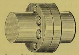
FIG. 4.—Safety Coupling with countersunk bolt-heads.
