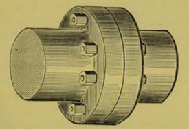
FIG. 3.—Coupling with dangerous projecting bolt-heads.
