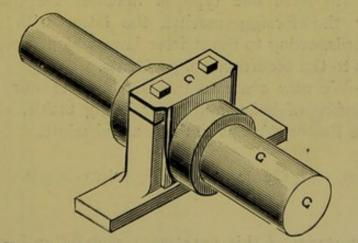
FIG. 13.—Shows a method of covering shaft ends with a sheet-metal cap (G).
