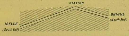
Fig. 75.—Section of Simplon Tunnel, showing difference in Levels between North and South ends.
