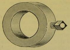
FIG. 5.—Collar with dangerous projecting set-screw.
