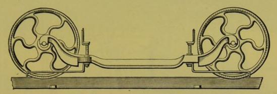
FIG. 20.—Hargreave's Mule Carriage Wheel Guard.
