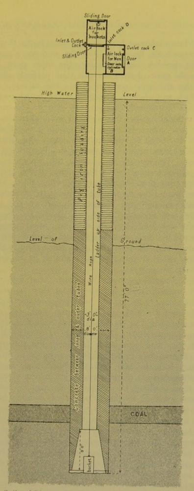
FIG. 73. -Section of Caisson used in rebuilding Redheugh Bridge, Newcastle-upon-Tyne.
