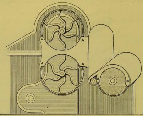
FI3. 10.—Incomplete guards for spur wheels. (The points of danger are marked A, A and B, B respectively.)
