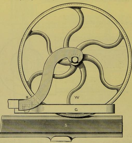
FIG. 19.—Self-acting Mules. Elevation—Foot-guard for carriage wheels. The guard (G) is fixed to the bracket (B), and surrounds the wheel (W) at a slight distance above the slip or rail (S).
