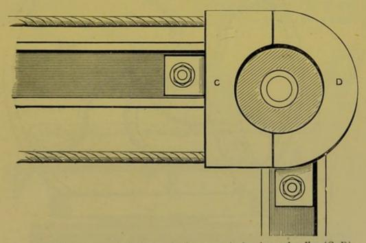
FIG. 18.—Shows a guard which completely covers the band round pulley (C, D).
