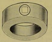
FIG. 6.—Collar with countersunk set-screw.
