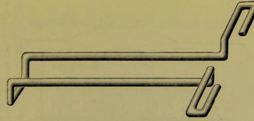
FIG. 21.-Hargreave's Mule Carriage Wheel Guard.
