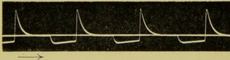
FIG. 38.—CURRENT CURVE OF SAME COIL, USING THE WHOLE SECONDARY COIL.
