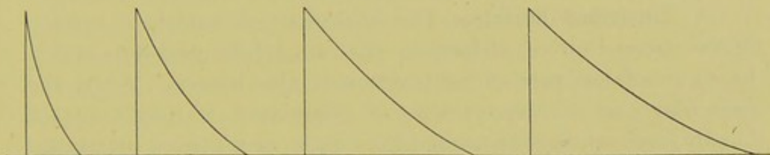
FIG. 158.—DISCHARGE CURVES OF CONDENSERS WHEN THEIR CAPACITIES ARE IN THE RATIOS OF 1, 2, 3, 4, WITH CONSTANT VOLTAGE AND CONSTANT RESISTANCE.
