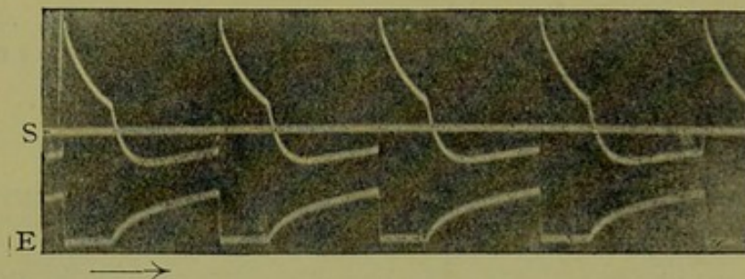
FIG. 36.—INTERFERENCE OF CURRENT WAVES WITH RAPID INTERRUPTIONS.
