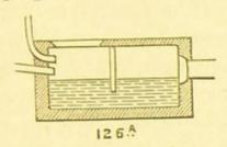
An attempt at ventilation is shown at Fig. 126a. What is radically wrong is the discharge of the sink pipes inside the trap, instead of above the gratings. With this exception this form is the readiest method of disconnection, when no iron or earthen-
