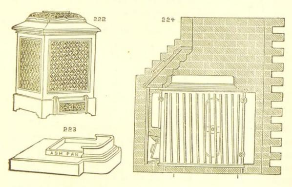
The design (Fig. 221) above is called the rough, slow combustion stove; but, where its plain appearance would be an eye-sore, the ornamental design shown at Fig. 222 is used, the cells being hidden by an artistic-patterned grating. For churches, these stoves are made with
