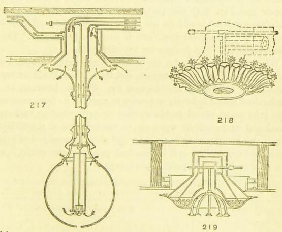
This paper would not be complete withou a description of the new ventilating globe light; therefore I give at Fig. 217 a section of that of Rickett's, manufactured by Messrs. Richardson, Slade, and Co.,
