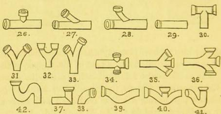
Fig. 26 is called the square single junction, Fig. 27 the oblique single junction, and Fig. 28 the curved single junction. They can be ordered by these names without any fear of mistake. The T-shaped junction Fig. 30, the Y-shaped junction Fig. 31, and the U-headed junction Fig. 32, are those used in diverting the heads of drains or in collecting two drains into one channel. The tapered pipe, Fig. 29, simply reduces a large-bored pipe to one somewhat smaller; Fig. 33
