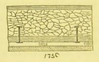
Fig. 175b represents the patent fire-proof system of Messrs. Fox and Barrett, of London. Here relled iron joists are substituted for the ordinary wooden joists, and are placed about two feet apart. Upon the bottom flanges of the irons are placed strips of wood, and upon these is laid the concrete, as shown. The floor may be laid of tiles, as in Fig. 175c, or joists of wood can be laid above the concrete and floor-
