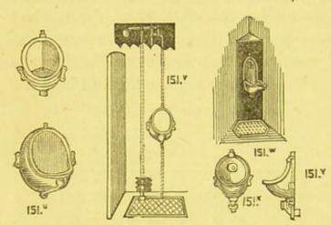
at the upper part of Fig. 151u. This has a perforated inlet pipe all round the top margin, by which means the whole surface is, or ought to be, washed. The lower sketch represents a 151. flat-backed receiver. At the lower part of both there is an outlet grating through
