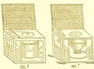
There remains a word to be said by way of conclusion about the portable water-closets. These are useful in cases of sickness, but ought to be used only in conjunction with the best disinfecting media, and should be immediately emptied
