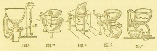
Underhay's regulator valve closet is drawn at Fig. 151*l*, and here no service box, cranks or wires, are at all required. A number of these closets can also be supplied from one cistern, and from any distance. The fixing is, moreover, excessively simple. At Fig. 151*m* may be
