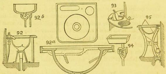
A very cleanly washstand slab, which drains the soap and brush trays, known as the Atlantic wash slab, is drawn in plan and section at Fig. 92a, and this costs, with patent plug and chain, a guinea. It is manufactured by Copeland and Sons, of Stoke upon Trent. At Fig. 92b is exhibited a washing sink with trap below, constructed entirely of glazed earthenware, and therefore rather a novelty. It is
