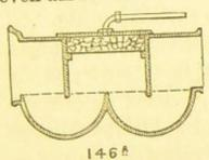
Not only were sewers fitted up as deodorents as time rolled on, but the benefits were soon extended to the traps of the house and stable. Fig. 146 gives an instance of this, and represents the present form of Mr. Cottam's efflurium trap, as fitted with a tray of oxidising material.
