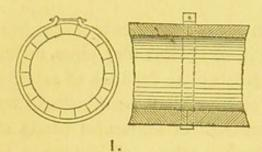
Some monster wooden drainage pipes, 3 ft. in diameter, built up in segments, 3 in. thick, and in 24 ft. lengths, 6 in. wide, have lately been manufactured in Gloucester. The joints are made with bands of iron 3 in. wide, tightened with a screw bolt, and these bands also occur
