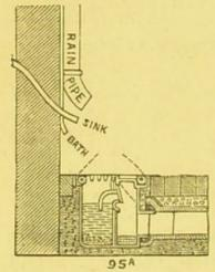
Waste pipes from the above-named places, and also all rain-water pipes should be led down to within 12 or 18 inches from the ground, and should deliver on to the grating of a gulley or yard trap, such as sketched at Figs. 99 or 102, p. 42. If needful, a larger yard trap can be used, such as shown at Fig. 95a., which is an adaptation of Fig. 109 p. 45; or if this is too small, an effluvium trap can be constructed of bricks and mortar, as
