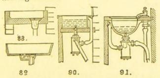
Although not long introduced the ordinary troughs and basins with plugs at the bottom and with supply taps, and the still newer ones with stop valve supplies, are sufficiently familiar as
