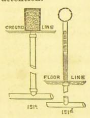
A novel system of rendering the drainage gases innocuous is sketched at 151c, and is the improvement proposed upon the underground trays by Dr. Taylor, of Anerley.
