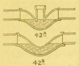
To revert for a moment to Figs. 39 and 40. I ought to point out that these are sometimes sadly abused. For instance, the former when laid in a drain, should resemble Fig. 42 b, and just exactly trap and no more. If too deep a syphon is used, it will speedily fill with sediment, as thousands of
