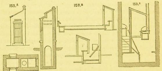
At Nottingham, some little time ago, the town Sanitary Committee established in some districts the ash closet, which is figured at 159a in the above group. As will be observed by the plan, elevation and section, a pit is formed, having watertight walls, under the whole closet. The floor of the pit below, which is also watertight, slopes on all sides towards the centre, so that the latest deposit of soil will be
