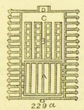
veloped gills, will be noticed at 229a, the invention of Messrs. Smith and Sons, of Barnard Castle, Durham. When the fire-box A is full of heated air and gases, they enter the tubes B. The letter C represents a smoke box, and the products of combustion are forced to pass through this before they escape by means of the stove-pipe D. The arrangement is mostly a repetition of some we have previously mentioned, but here the gills,
