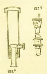
At Fig. 159q is given an illustration of the overflow trap, supplied by Mr. Finch, of High Holborn. It is in principle the same as the Antill trap, shown at Fig. 80, page 36. The other design, Fig. 159p, represents the patent overflow arrangement of Messrs. Westo and Pinder, sold at Eaststreet, Walworth, London. Here an inverted cup is fitted on the bottom of the outer overflow pipe. The inside of the regulator is made to contain some soft filtering material, such as wool or
