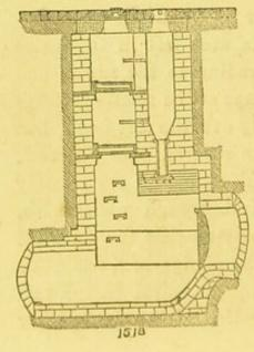
Fig. 151a represents the usual method of ventilating and deodorizing pipe drains, and here the charcoal screen is placed vertically in the partition between the manhole and the smaller ventilating chamber. I copy this figure from the "Suggestions relative to Sewage," prepared by Mr. Rawlinson in 1867.
