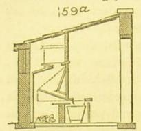
I give at 159a, and which has received great commendation. Through the opening in the back or lower wall the unscreened ashes are thrown, and pass through a screen into the hopper below. When the closet is used the seat is depressed, and this in its turn imparts a shivering motion to the screener, which serves the purpose of sifting the cinders from
