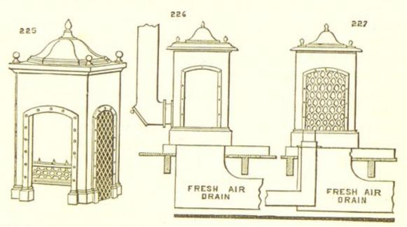
At Fig. 225 will be noticed what is called the patent pyro-pneumatic stove grate, made upon the principle that fire-lumps are the best and purest media for the transmission of heat by radiation.
