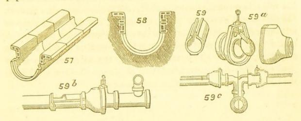
I will here describe the patent open channels and flanges of Messrs. H. Doulton and Co., of Lambeth, which have been specially contrived for sewerage, irrigation, and for use in sewage farms. The channels or gutters are of earthenware, and these are glazed, as it has been found that not only ditches and rough conduits of bricks, but also unglazed material, harbour vegetable growths and impede the flow of the liquids, not to mention the incessant labour of cleansing them out.
