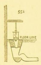
An attempt to obviate the necessity of disconnection of the sink with the drain is exhibited at Fig. 95b, and is the invention of Dr. Taylor, of Anerley. A shallow sink is here furnished with an ordinary bell trap at the upper end of the waste pipe, and the other end of the waste pipe is turned up to act as a syphon. This last portion is enclosed in a valve box, which contains a float or valve somewhat resembling
