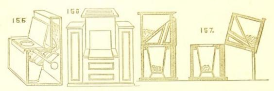
being panelled throughout, and also made with an easy slope to the Fig. 156 shows a closet of this description for indoor use, made to resemble a chest of drawers, when the top flap is pulled down upon the seat. The earth hoppers are in the wings. He also sells a cheap out-door closet, made for fixing over a pit, either single or in rows, being in fact a skeleton apparatus. The whole are made self-acting.
