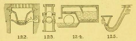
There is a peculiar system of self-acting trap, which I draw at Fig. 122; but it has not been used of late years, owing to the introduction of better kinds. It is said to have acted in places where the gully well was not deep, and where the scoop, when falling, would immerse itself in water. Supposing the mud scoop to be choked, in that case the water would fill up the body of the trap; but when two-thirds full of water, the weight of the mud and superincumbent fluid
