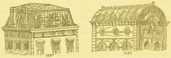
and would suit the majority of cases very well. The construction of the roof-garden conservatory would not, necessarily, differ much from those built on the ground. The most elegant kind of roof for the purpose, would, perhaps, be the wood and glass roof introduced by Mr. Cranston, of Birmingham. An iron and glass construction, very suitable, would be that known as Ayre's Patent, manufactured by the Imperishable Hothouse Company, of Newark-upon-Trent. The
