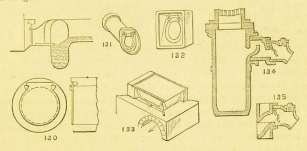
Figs. 131 and 132 represent the present forms of valve traps, and as made by nearly all the earthenware pipe-makers. Each manufacturer's trap has its individuality, which lies in the mode of hanging the flap, and all kinds are more or less effective. Where stoneware is used, the surface is ground. The flaps are now made of galvanized iron, fitted sometimes with gun-metal eyes, (in the manner shown at Fig. 131,) and at other times with chain rings, as drawn at Fig, 132.
