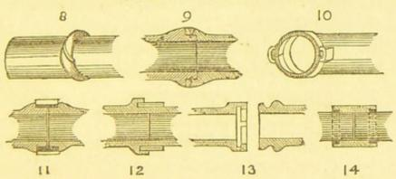
With reference to the jointing of these pipes at Fig. 8, may be noticed what is called the half-socket pipe, and this is a form very
