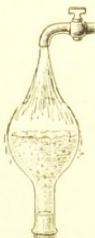
Fig. 81.—Water boiling under reduced pressure.
