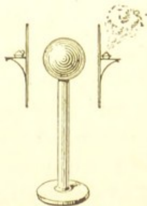
Fig. 73. — Absorption by black and by polished plate.
