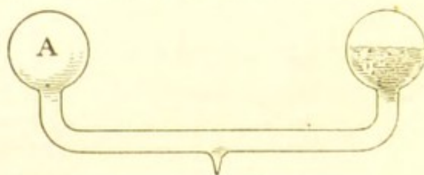
Fig. 82.—Ether boiling with the warmth of the hand.
