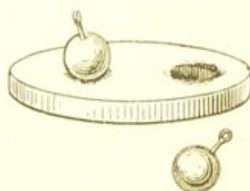
Fig. 95. — Greater heating power of iron compared with bismuth.
