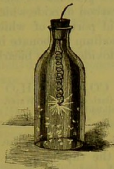
Fig. 7.—Combustion of Steel-wire in Oxygen.
