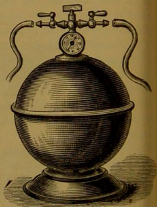
Fig. 17. Compressed-air cylinder, with air-gauge, etc.
