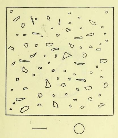
Sketch of larger particles of silica isolated from silicotic lung. × 1,000.
