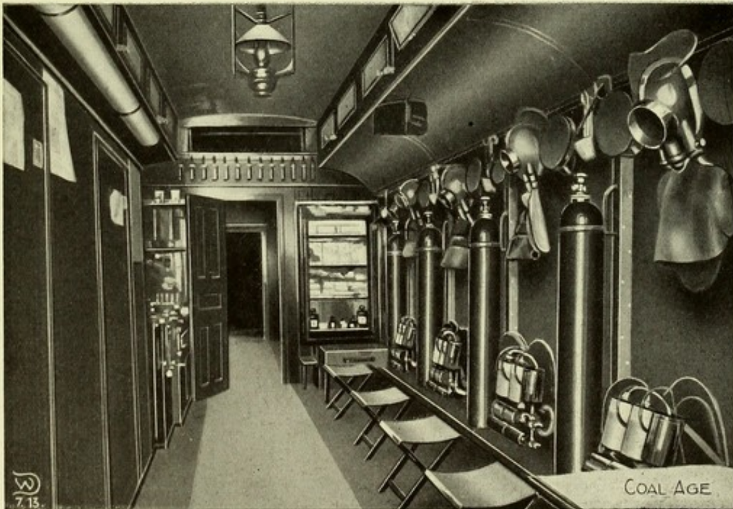
Fig. 7. Rescue-Car of the Nova Scotia Steel and Coal Company (Canada) equipped with Draeger Rescue Apparatus and Pulmotor.
