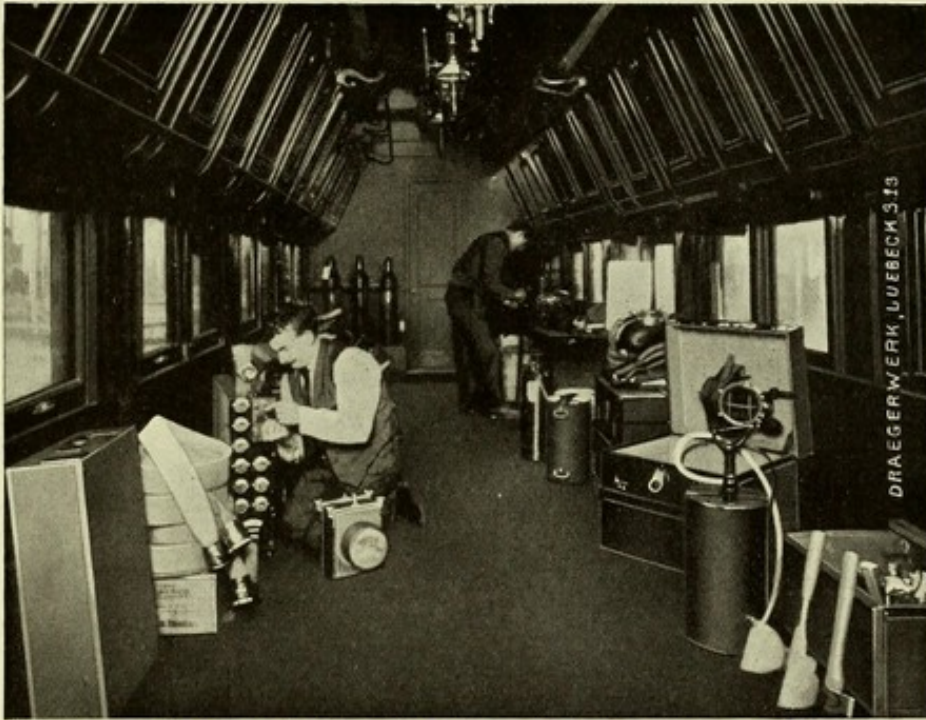
Fig. 6. One of the 7 Rescue-Cars of the U. S. Bureau of Mines, equipped with Draeger Apparatus.
