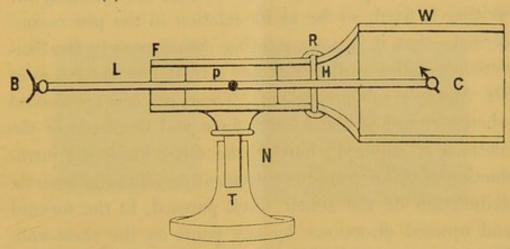
A writing-frame (w) is attached to the instrument by a hinge (H); and a spring (R) keeps it continually pressed against the pencil at c. The whole mechanism is then allowed to rotate upon the pivot (N) in the stand (T).
