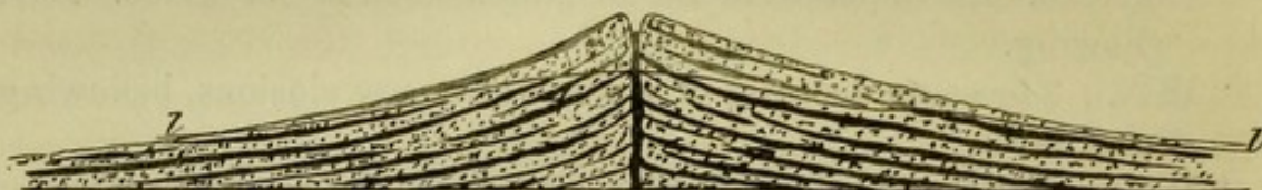
FIG. 1.—Diagram section of a volcano. The dark bands represent lava-streams; the dotted spaces, ashes and scoriæ; and the line l , the water level in the mountain.
